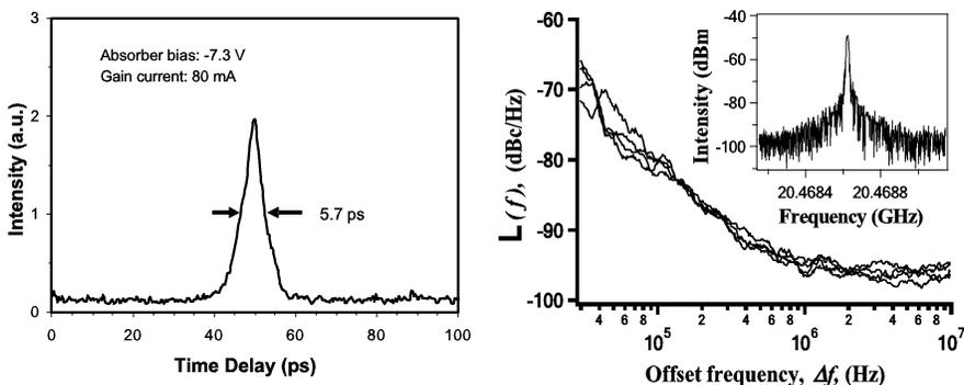
Fig 2. The autocorrelation signal and the single-sideband phase noise spectral density  $L(f)$  of the 2-section QD passively MLL shown in Figure 1. The inset is the ESA spectrum of the 4<sup>th</sup> harmonic. The bias condition is:  $I_g = 80$  mA and  $V_a = -7.3$  V. Optical pulses with pulse width of 5.7 ps and RMS jitter of 0.91 ps at a 5.17 GHz repetition rate were obtained.
