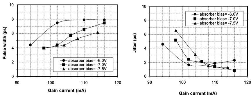
Fig 3. The pulse width (left) and jitter (right) of a 1310 nm QD passively MLL as a function of the gain current and absorber bias. An operation window of >15 mA in gain current at absorber bias from 6 to 7.5 V was obtained, leading to pulses with <10 ps pulse width and <3 ps RMS jitter.
