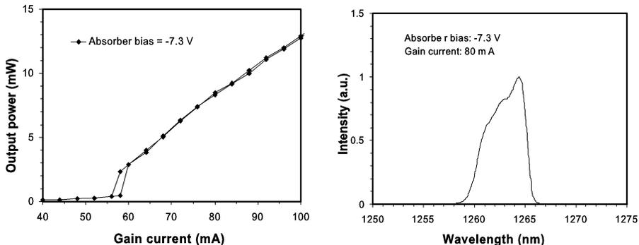
Fig 1. The CW L-I characteristics and optical spectrum of a 1250 nm QD passively MLL under absorber bias of -7.3 V.
